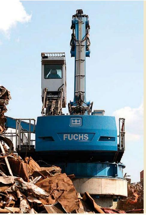
Wherever excellent loading performance and continuous availability matter, stationary loading machines from TEREX Fuchs offer an optimal solution for the feeding of processing systems like scrap shears, scrap presses or shredders.
